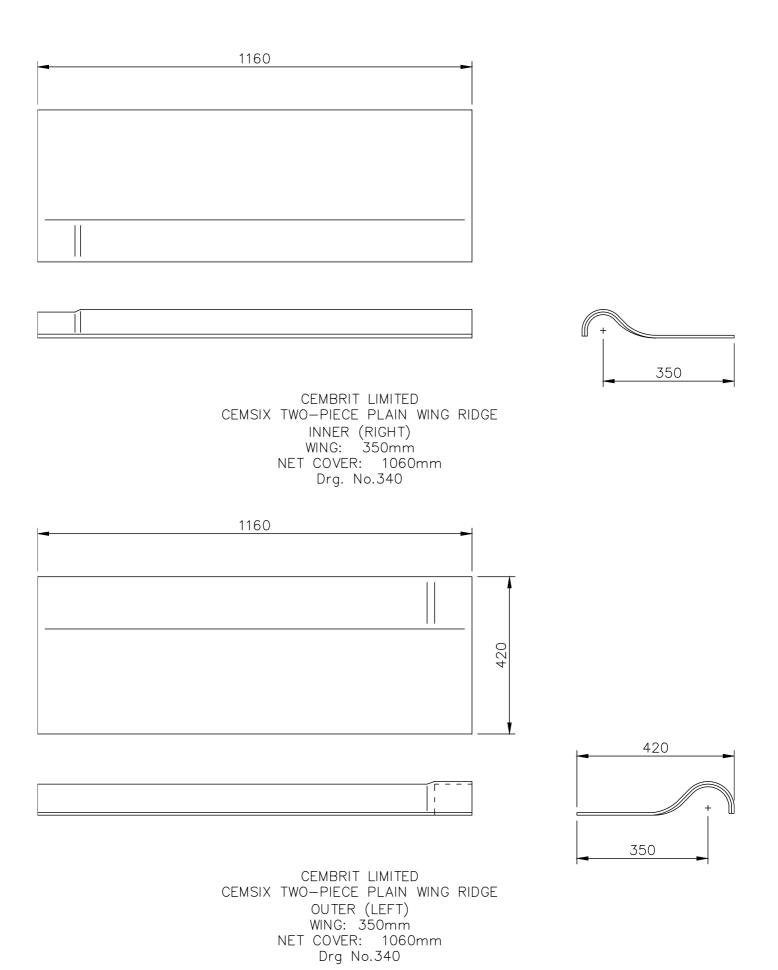
FOR ROOF PITCHES BETWEEN 5° AND 15°, IT IS NECESSARY TO TRIM THE ROLL OF THE OUTER RIDGE WING ON SITE TO CLEAR THE CORRUGATED PORTION OF THE INNER RIDGE WING ALONG THE LENGTH OT THE RIDGE
